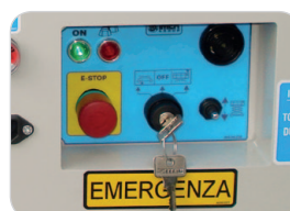
Ground control panel, intuitive and well protected from accidental bumps.
