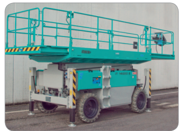
Large working surface with double deck extension (total: 14 sq.m.). Access by lateral double ladder.
