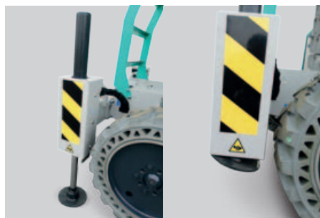
Automatic hydraulic stabilization system
