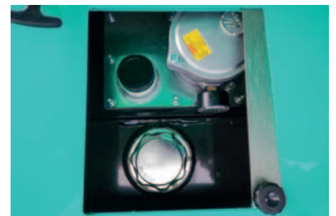
Sliding opening for filling fuel without the need to open the side hood
