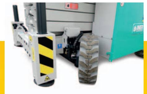
Reduced steering angle thanks to 70° wheel inclination
