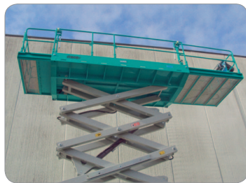
Manual double asymmetric deck extension (2 m front + 0.9 m rear).
