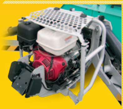
Engine guard enable high accessibility and impact's protection
