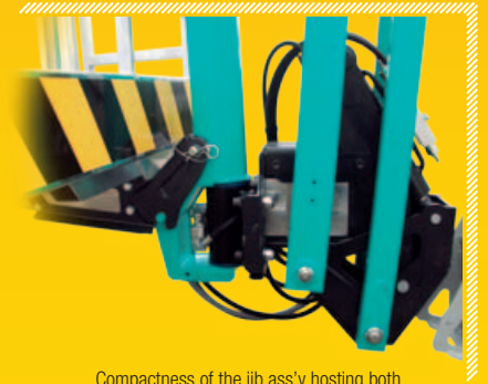
Compactness of the jib ass'y hosting both the load cell and basket rotation system.
