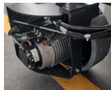
AC electric motor. 90° wheel steering.
