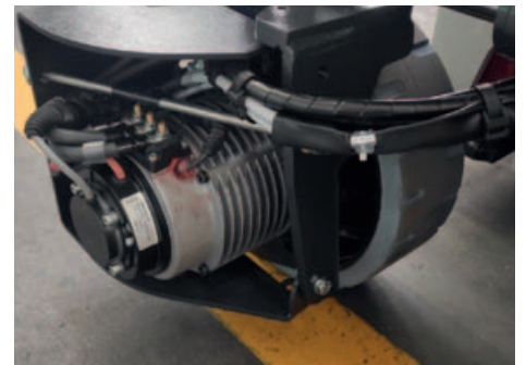
AC electric motor. 90° wheel steering.
