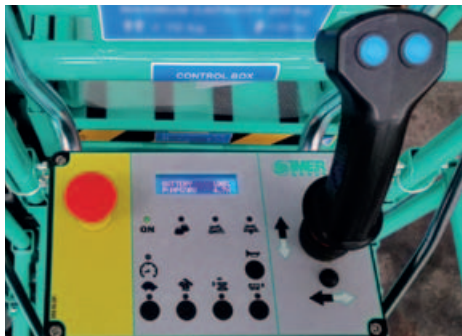
Control panel on the platform with capacitive buttons: simplicity and safety of use.
